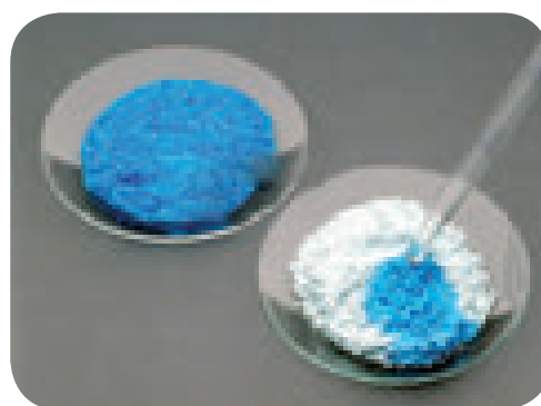
Figure 9.10 Anhydrous copper sulphate turns to blue when water is added
